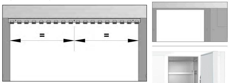
Step 2: Fix the suspension rail using the three mounting screws. After fixing the first screw make sure that the suspension rail is perfectly leveled.
