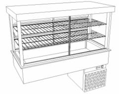
Refrigerated **basin** curved on all sides for easy cleaning; insulated with condensation drained to removable container; temperature attainable in basin +4°/+10° C.
