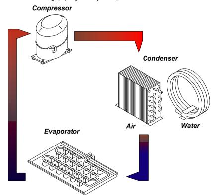
Each ice maker uses the properties of compression and expansion of the liquefiable gases; its main principle is that each change of bodies state is got by producing or absorbing heat.
