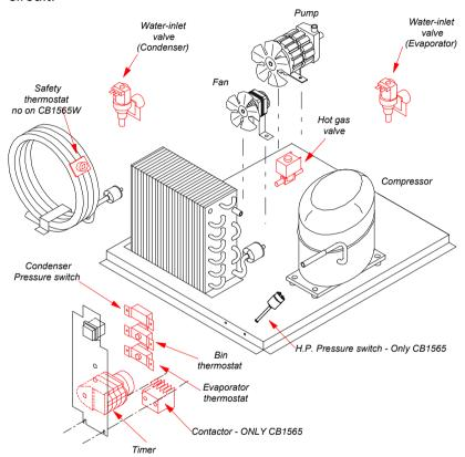
The ice maker is energized by the bin thermostat, that stops machine when the bin is full.
