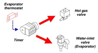
The pump is stopped and also the spray noozles stop; on the contrary, the hot gas valve is started in order to pipe the refrigerating fluid (overheated) directly to the evaporator.
