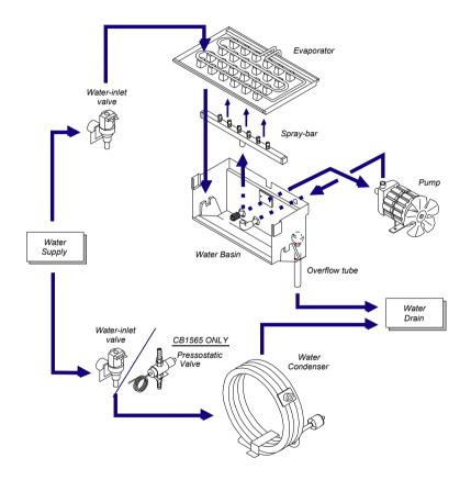
The water supply circuit of the basin, the water-inlet valve, the pump and the evaporator are on all machines of the 'CB'-line; the water condenser circuit, on the contrary, is on water-cooled versions only.
