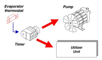
Some minutes after the beginning of the ice production phase, due to the refrigerant in expansion in the coil, an ice layer starts to form inside the cups; the evaporator thermostat, perceiving a drop in temperature of the evaporator, starts the timer, in order to complete the ice production phase.
