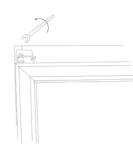
8. Tighten the top hinge pin.
