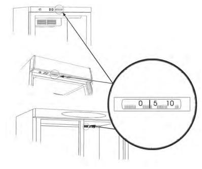
Depending on model the thermometer can be placed as follows:
