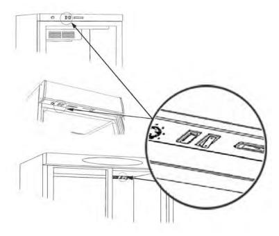
Appliance with internal light has a light switch. Depending on model this is placed as follows:
