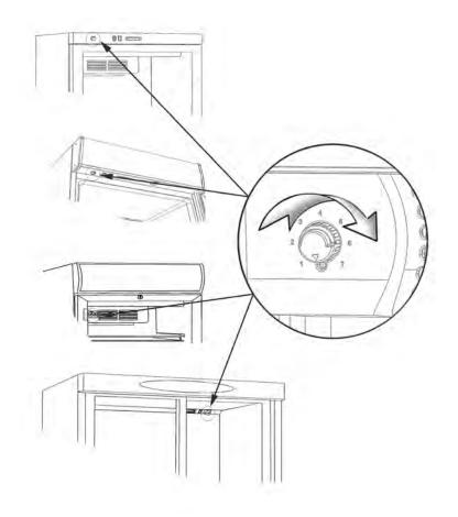
Depending on model the thermostat can be placed as follows:
