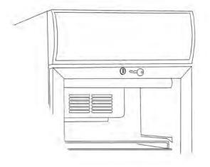
The appliance with hinged door has a lock. The lock is placed at the top of the door.
