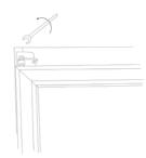
8. Tighten the top hinge pin.
