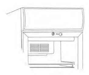
The appliance with hinged door has a lock. The lock is placed at the top of the door.
