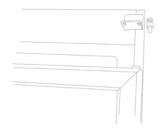
5. Remove the top hinge pin.
