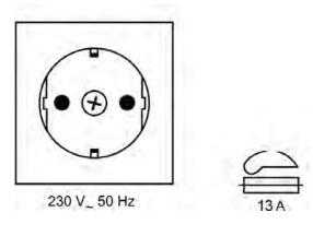
The appliance should be connected to an 13A protected socket.
