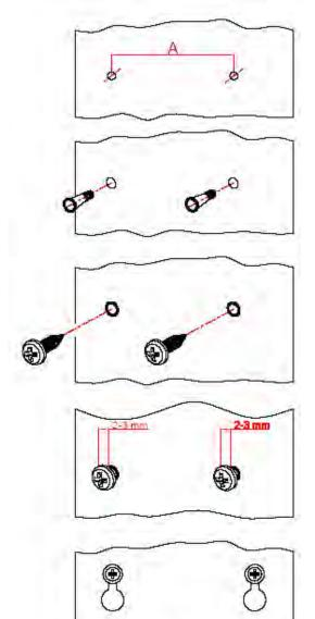
Drill 2 holes with a diameter of 8 mm and a depth of 40 mm and a distance as shown on the drawing (A).
