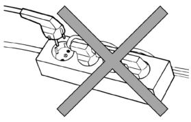
The appliance should not be connected to a multipoled distribution socket.
