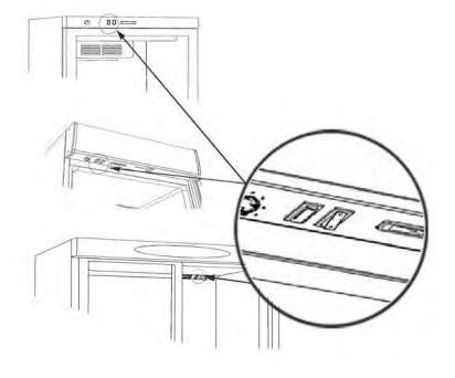
Appliance with internal light has a light switch. Depending on model this is placed as follows:
