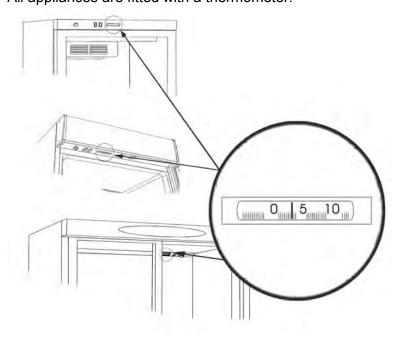
Depending on model the thermometer can be placed as follows:
