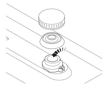
The presence of dirt inside the appliance can obstruct the nozzles, and thus affect the flame.
