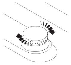
Before lighting the burners make sure the flame spreaders are turned to the stop position.
