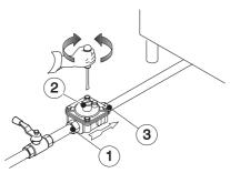
**AUSTRALIA:** the gas pressure regulator supplied with the appliance must be fitted to the appliance inlet. Adjust the test point pressure with all hob burners operating at maximum setting as follow:
