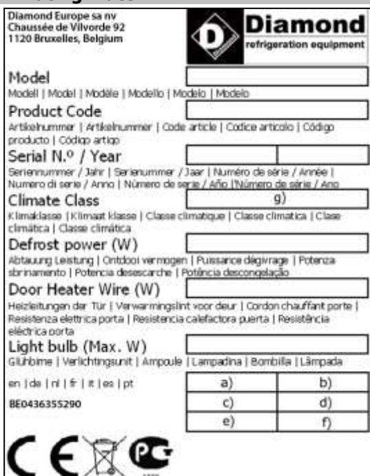
The rating plate on our equipment is located inside the equipment, on the left side panel. It includes the main technical data about the equipment and it identifies the MODEL and SERIAL NO., which are vital pieces of information for any queries to the manufacturer.
