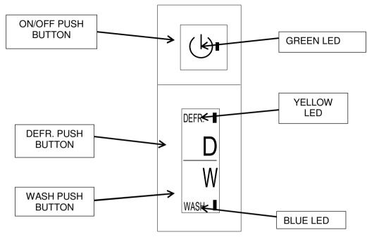
ON/OFF PUSH BUTTON: DEFR. PUSH BUTTON: WASH PUSH BUTTON: used to turn on and turn off the appliance - GREEN LED allows to start the defrost cycle - YELLOW LED allows to start and/or finish the washing cycle - BLUE LED.
