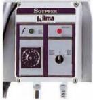
Low voltage control board (24 V.) equipped with: ON/OFF push button, manual/stop/automatic selector, flow programmer, power indicator and faulty connection light. Protection degree: IPX4.
